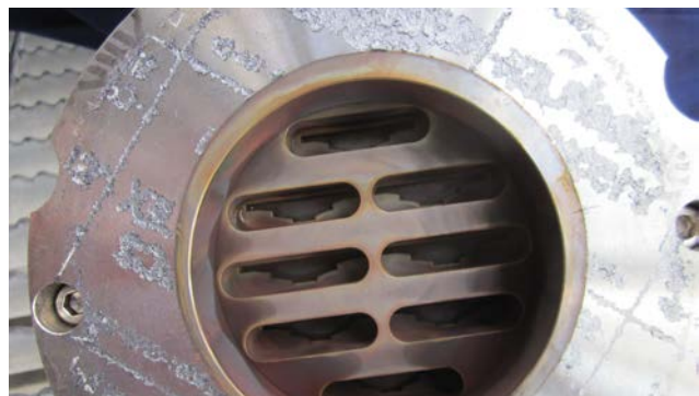
Fig. 7 The valve was dismantled after 1 year and no damage whatsoever and examined.
